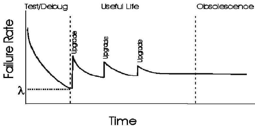
Figure 2. Revised bathtub curve for software reliability
