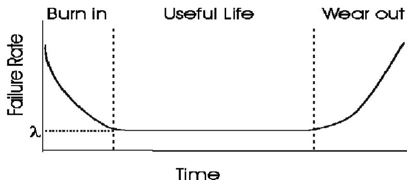
**Figure 1. Bath tub curve for hardware reliability**
